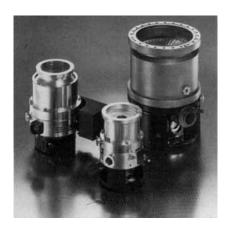
The V-versions (vertical) are designed for upright installation only, while the H-version (horizontal) can be incorporated between the vertical and horizontal. With a modification kit the V-version can be converted at a later time for horizontal use.
